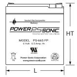
L: 3.86 (98) W: 2.20 (56) H: 3.78 (96) HT: 4.02 (102) Tolerances are +/- 0.04 in. (+/- 1mm) and +/- 0.08 in. (+/- 2mm) for height dimensions. All data subject to change without notice.
